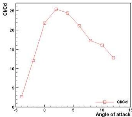
Fig. 4-19 lift-drag ratio curve
