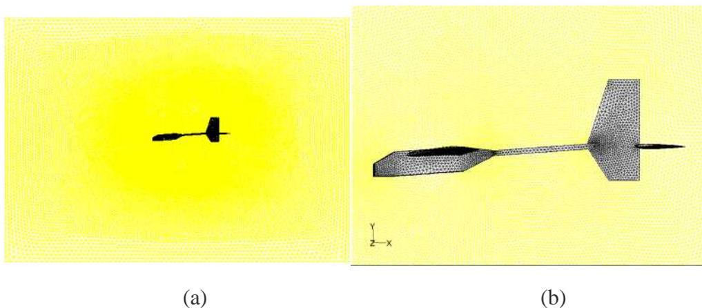
Fig. 4-2 mesh of the aircraft
