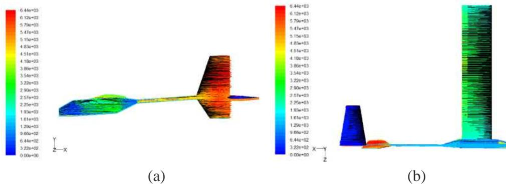
Fig. 4-13 oil flow distribution at 0° angle of attack
