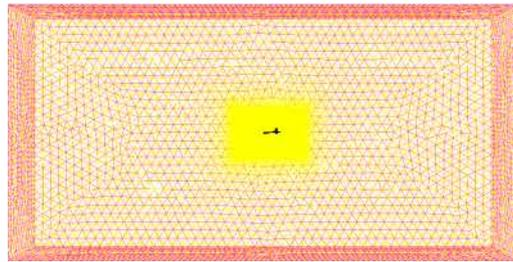
Fig. 4-1 mesh of the aircraft and the outer flow field
