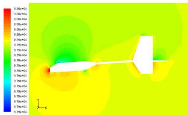
Fig. 4-12 pressure distribution at 12° angle of attack
