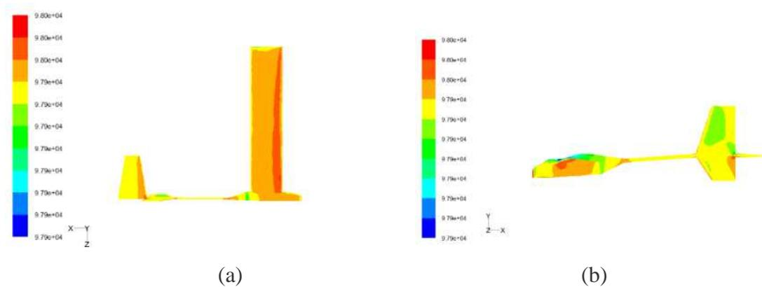
Fig. 4-11 pressure distribution of the plane surface at 12° angle of attack
