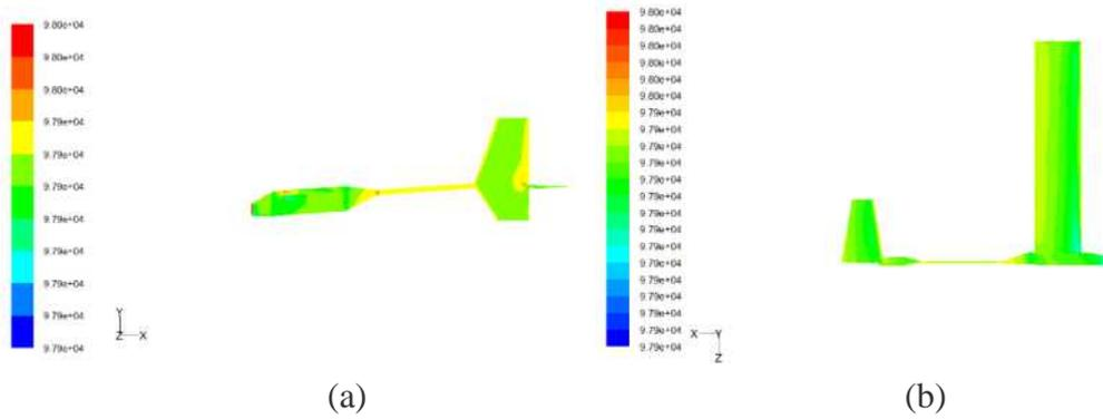
Fig. 4-3 pressure distribution of the plane surface at  $-4^\circ$  angle of attack
