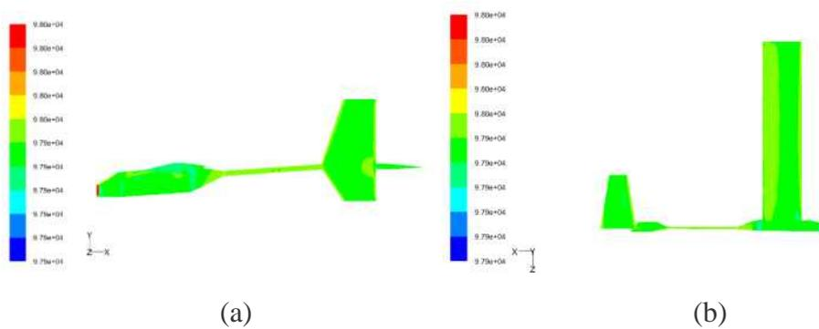
Fig. 4-5 pressure distribution of the plane surface at  $0^\circ$  angle of attack
