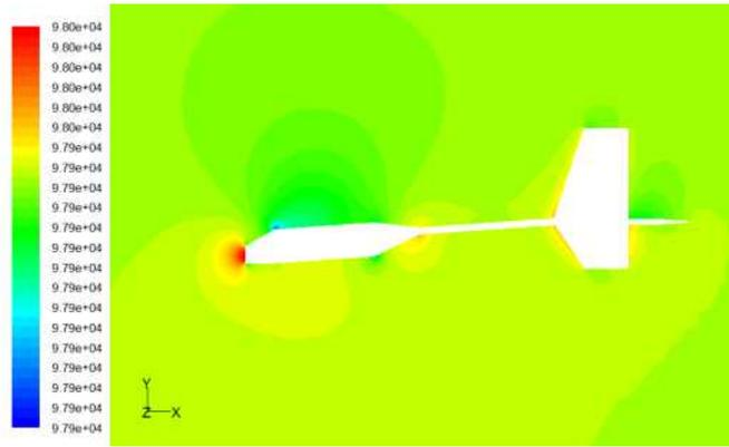
Fig. 4-10 pressure distribution at 12° angle of attack
