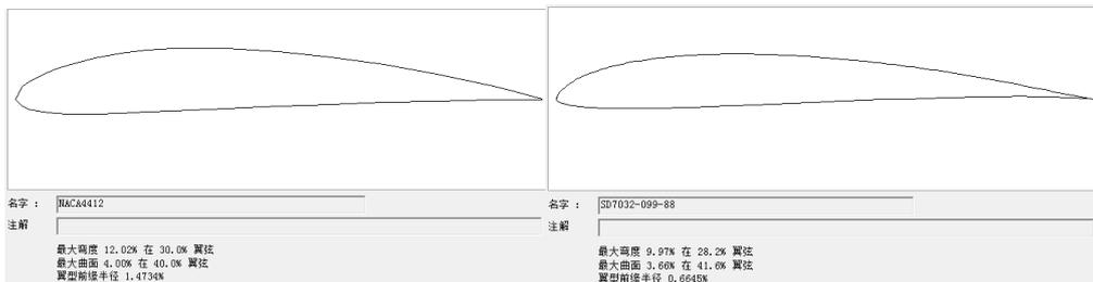
Fig. 3-10 NACA4412 airfoil
