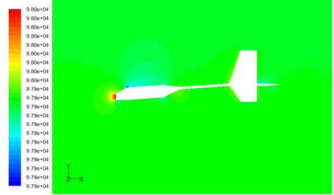
Fig. 4-8 pressure distribution at 4° angle of attack
