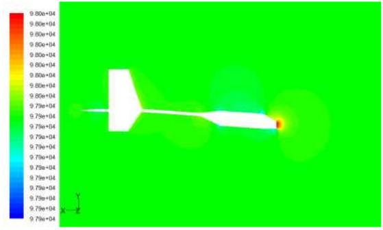
Fig. 4-6 pressure distribution at 0° angle of attack
