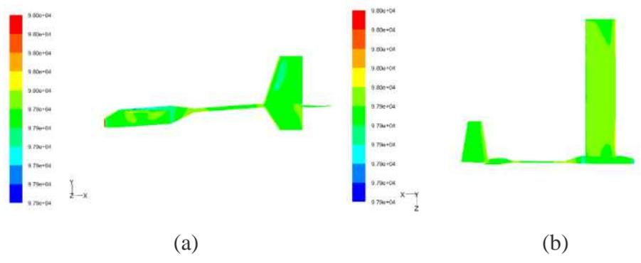
Fig. 4-7 pressure distribution of the plane surface at 4° angle of attack
