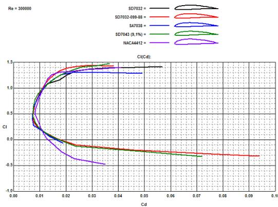
Fig. 3-12 CI-Cd curves of 5 airfoils when Re=300000
