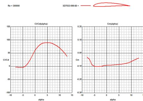
Fig. 3-13 the lift-drag ratio of SD7032-099-88 when Re= 300000
