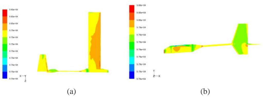
Fig. 4-9 pressure distribution of the plane surface at 8° angle of attack
