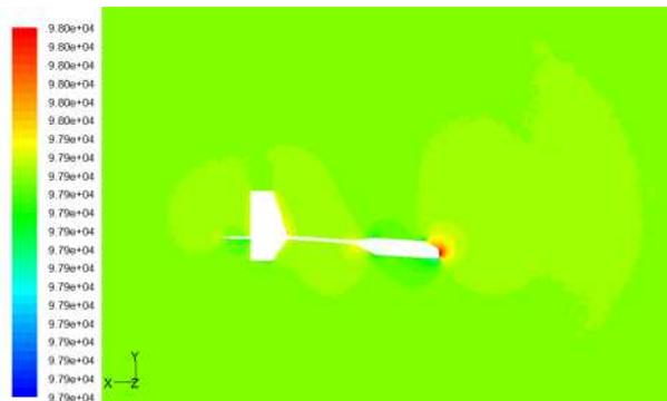
Fig. 4-4 pressure distribution at  $-4^\circ$  angle of attack
