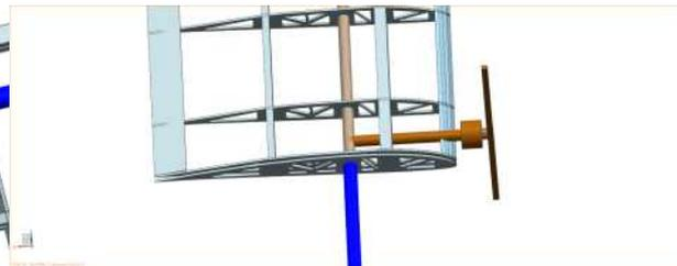
Fig. 3-17 rotating part of the wing
