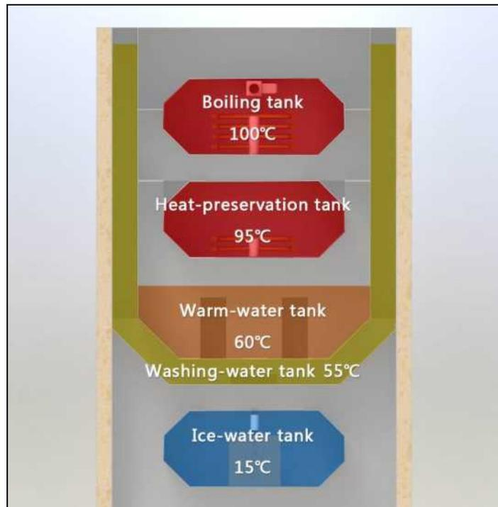
**Figure 3.1 The temperature distributed diagram of tanks**
