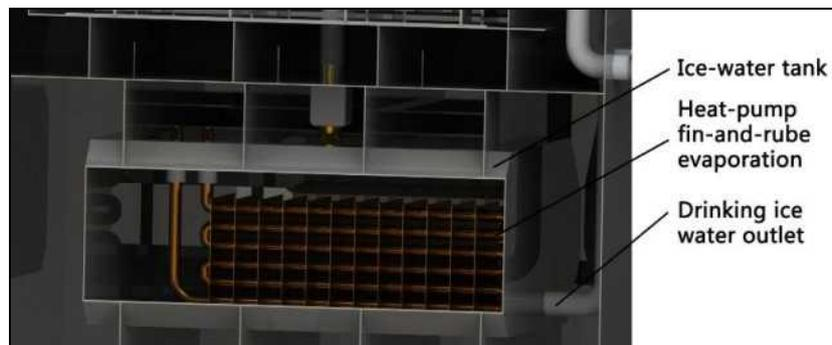
Figure 2.4 Internal structure of the ice-water tank
