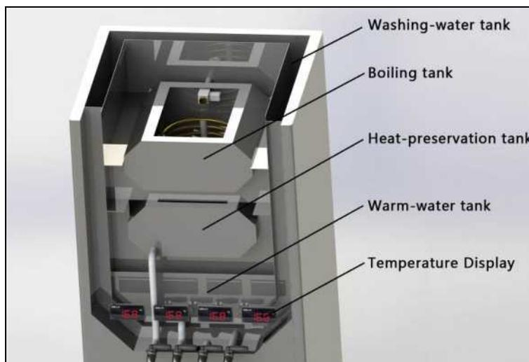
Figure 2.2 The internal structure feature without head cover
