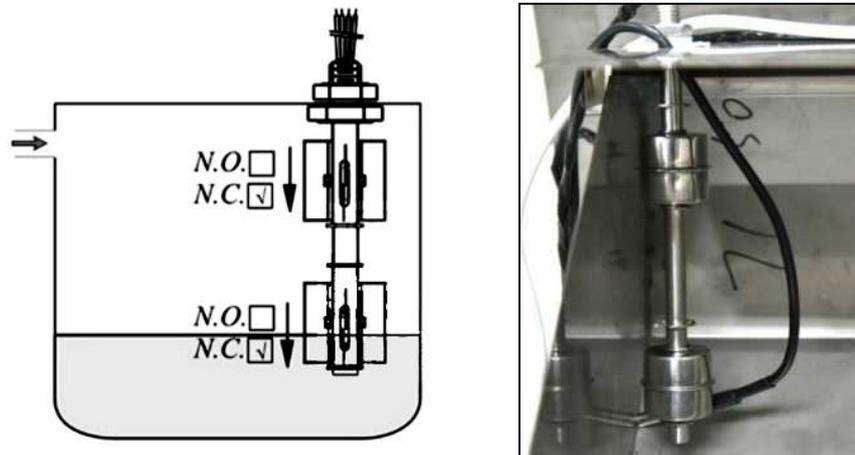
Figure 2.9 The Schematic and installation effect of double float switch
