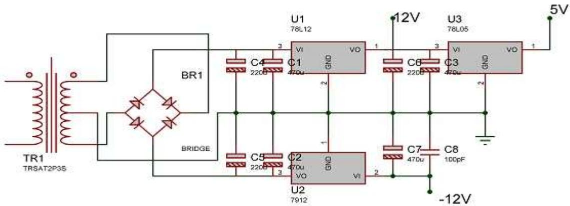
Figure 2.6 The circuit diagram of the power conversion section
