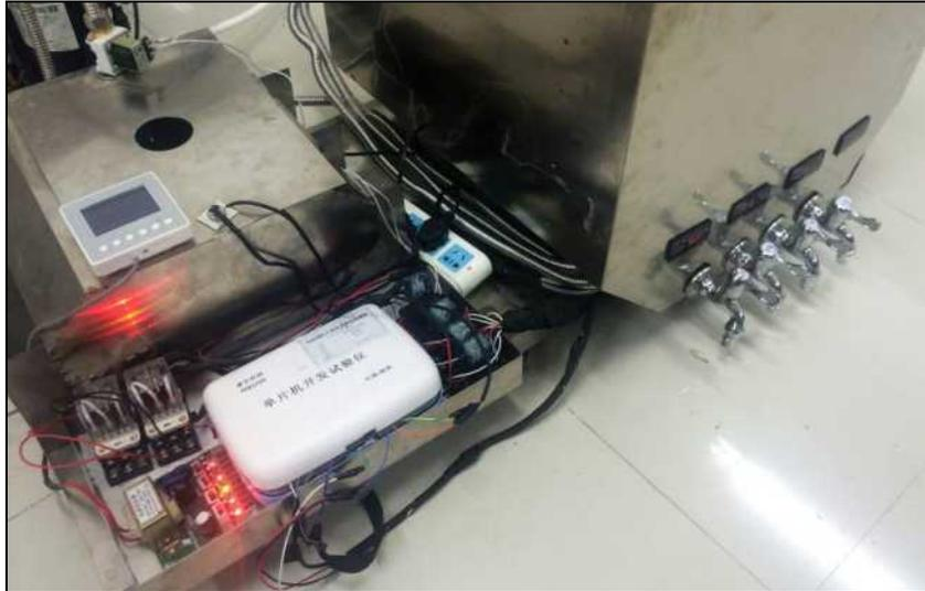
Figure 5.2 Electronic control systems and electromagnetic relay
