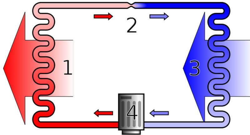
Figure 3.2 A simple stylized diagram of a heat pump's vapor-compression refrigeration cycle
