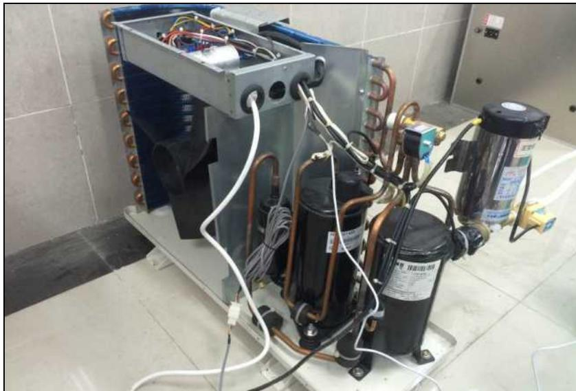
Figure 5.3 Air-source heat pump of the water boiler
