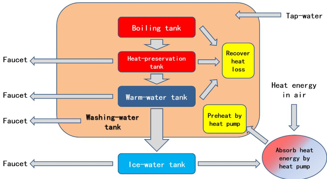
Figure 3.3 Work flow chart of the heat pump
