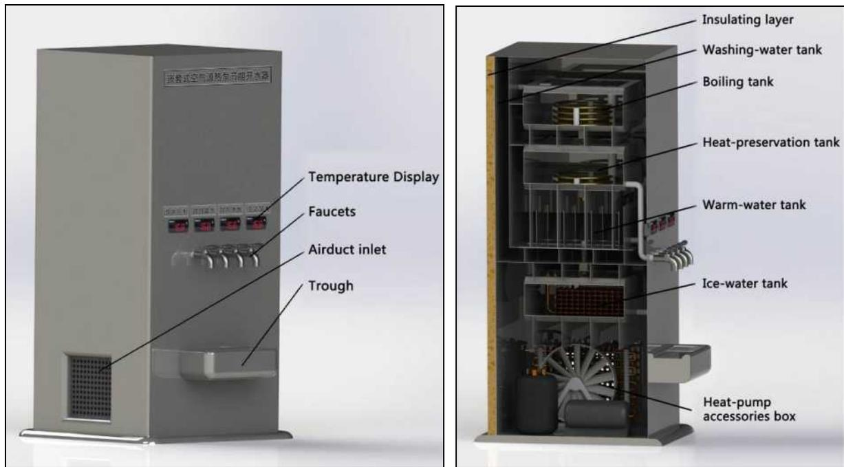
Figure 2.1 Front view and section view of the nested energy-saving water boiler
