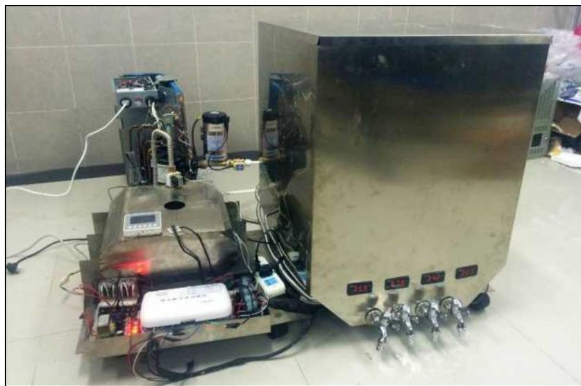
Figure 5.1 The nested energy-saving water boiler
