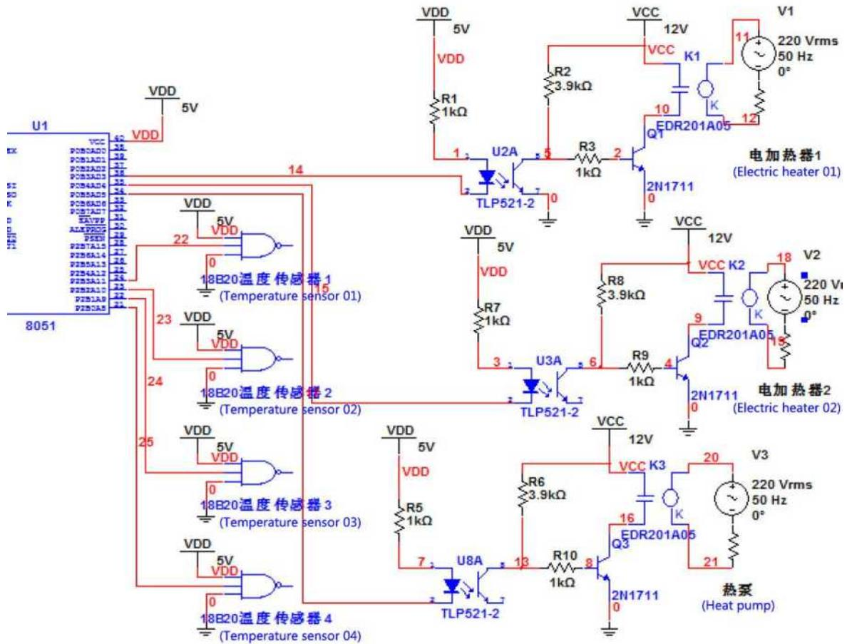
Figure 2.7 The circuit diagram of the temperature control section
