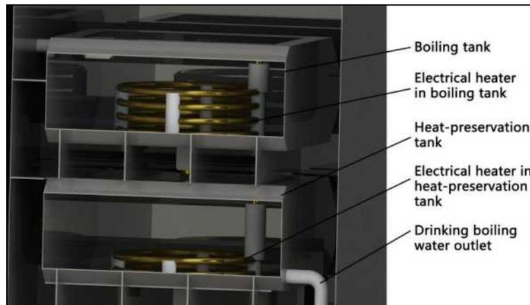
**Figure 2.3 Internal structure of the boiling tank and the heat-preservation tank**
