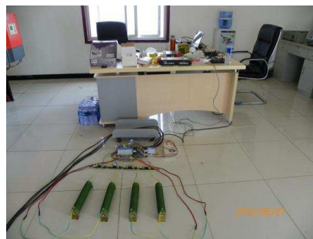
Figure 5. The measurement system of PV module output
