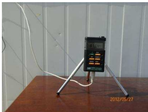
Figure 4. Radiation meter for the solar radiation
