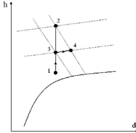
Figure 7 Enthalpy wet figure of the heating processes of the cooling air
