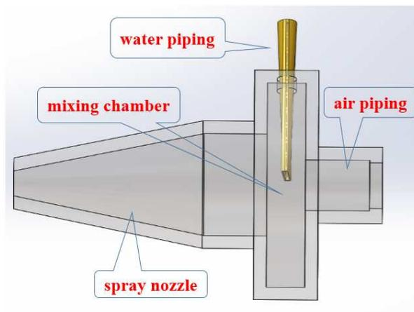
Figure 6 schematic diagram of spray nozzle
