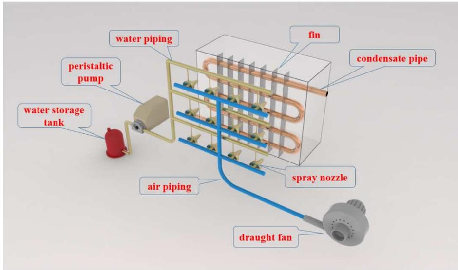
Figure 5 the overall system diagram
