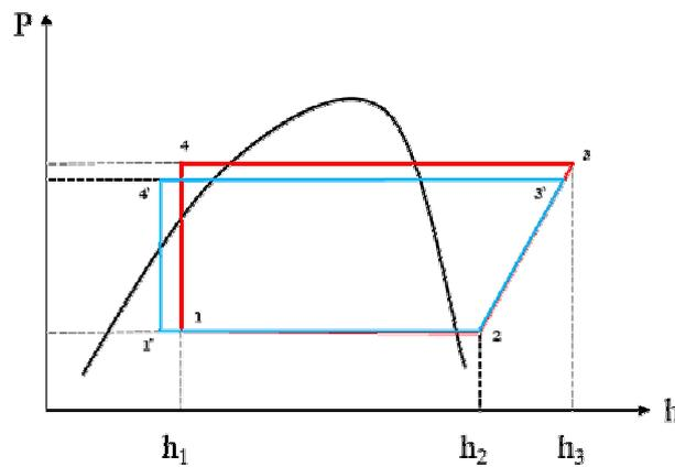
Figure 8 Refrigeration cycle comparison before and after adding spray
