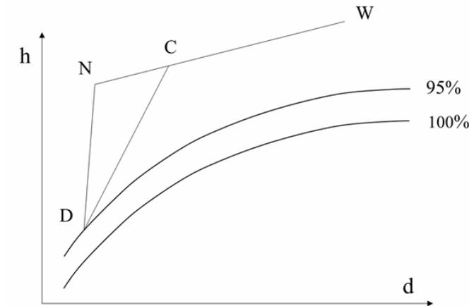
Figure 1 the psychrometric chart in the air treating process
