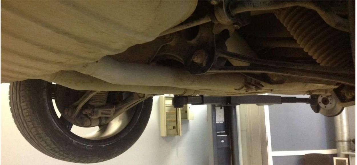
Fig. 3. The muffler has a slope down to the front of the car (AudiQ7 / 4LB / 2012)
