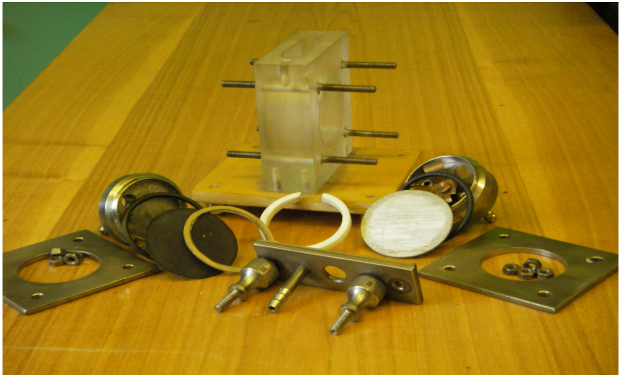
Picture 3. Structure of the laboratory thermo controlled aluminium-air cell
