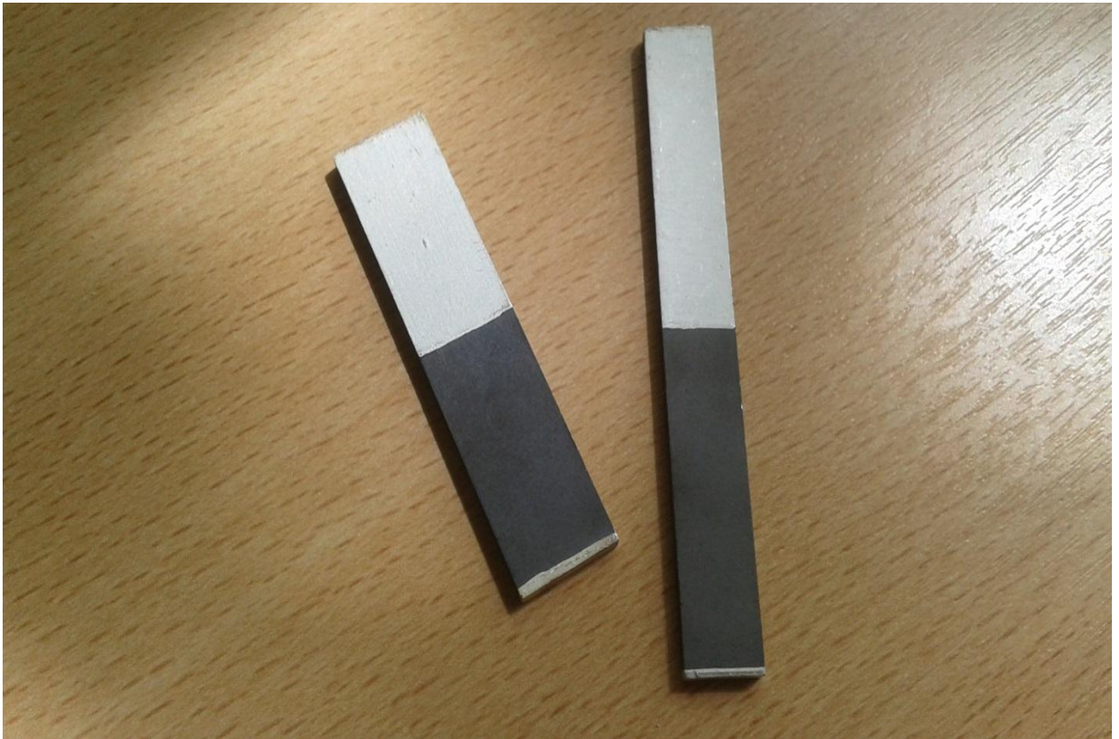
Fig.1 Piezotransformers with autoelectronic emission
